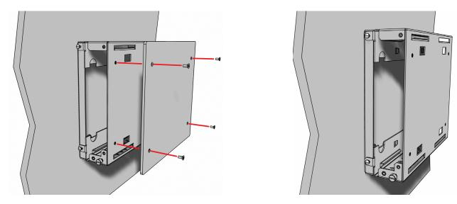
Figure 3. Cover Plate Removal
